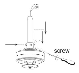
(3) Install in order the yoke cover, Canopy, Hanging Ball on the installed Down rod. slide Hanging Ball down to expose the hole, put the fixing pin into the hole, slide the Hanging Ball up and turn it left and right, let the fixing pin enter the Hanging Ball card slot.
