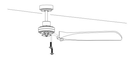
Remove the pre-installed screws.
