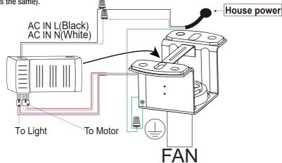
2) Put the receiver into the Bracket and arrange the wires
