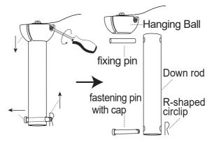
2 Pass the cable through the down rod and lock the down rod.
