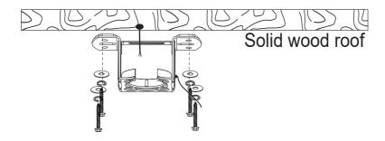
(3) Snap the basically assembled fan into the installed Bracket.
