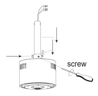
3 Install in order the yoke cover, Canopy, Hanging Ball on the installed Down rod. slide Hanging Ball down to expose the hole, put the fixing pin into the hole, slide the Hanging Ball up and turn it left and right, let the fixing pin enter the Hanging Ball card slot.
