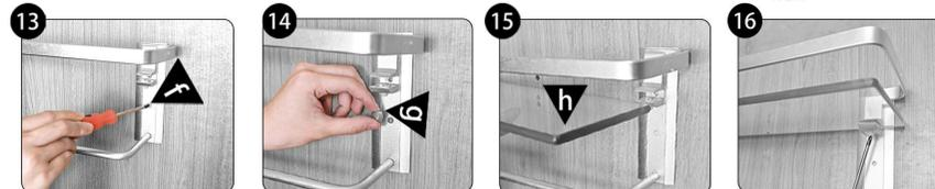
13. Use "f" to fasten the bracket to the wall
