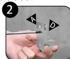
2. From the backside use the screw which take off from D to fasten "A", "D"
