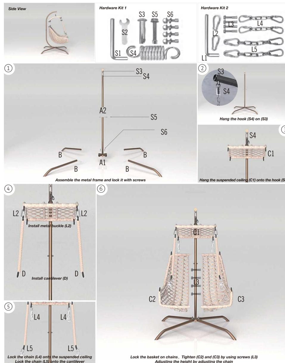
Use A Small Wrench Or Hexagonal Screwdriver To Tighten The Screws.
