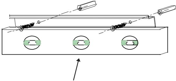
Draw horizontal line connecting the two bottom marked location. the line should to be level. adjust to level if necessary.
