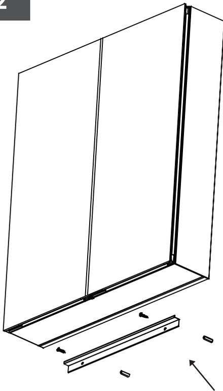
Attach the bottom mounting bar hanger to the wall with two mountin screws from the hardware pack.
