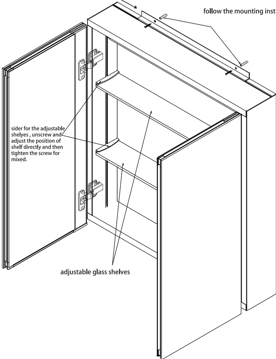
Put the cabinet on the bottom bar hanger and hold the cabinet, please make sure that the hanger must mach the track from the bottom board of the cabinet
