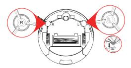
Please install the right brush into the right bottom mounting port of the machine, the left brush into the left botom mounting port of the machine, andensure that the two side brushes are in place.
