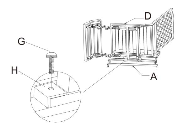
STEP 3: Attach the left arm (B) to seat panel using washers (H) and bolts (G). Please do not fully tighten all bolts until unit is fully assembled.
