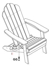
8. Lay the cup holder I flat, insert the bolt GG into the hole of the cup holder from bottom to top, and finally insert it into the hole on the back of the armrest and fix it.
