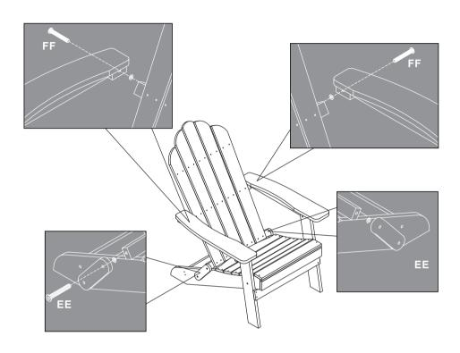
7. Insert the bolt EE into the other hole of the part E, then insert the washer into the end of the bolt, and finally insert the bolt into the hole at the lower end of the backrest and fix it.
